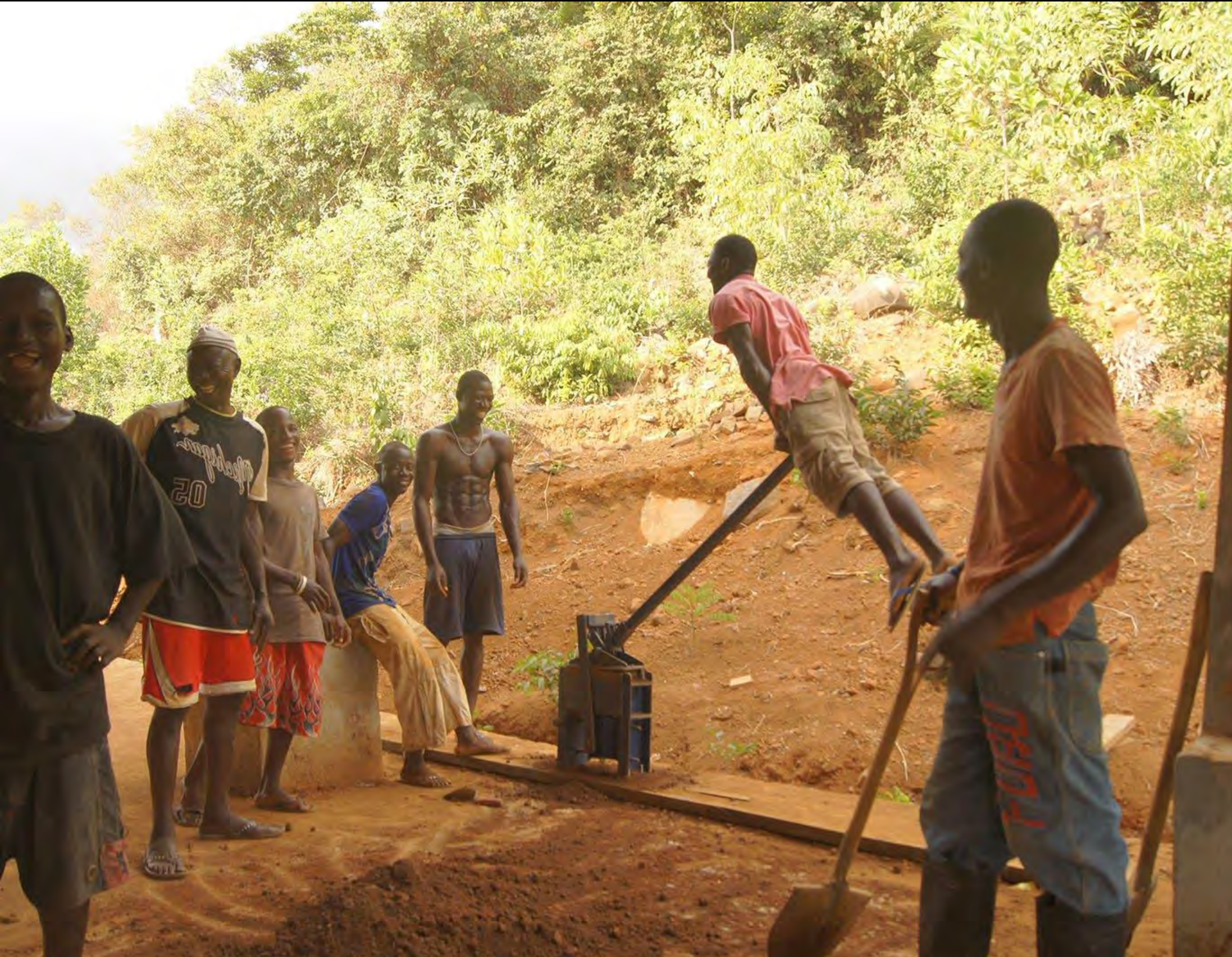
SOIL PRESS LOCAL SOIL PRESSED TO BRICKS
